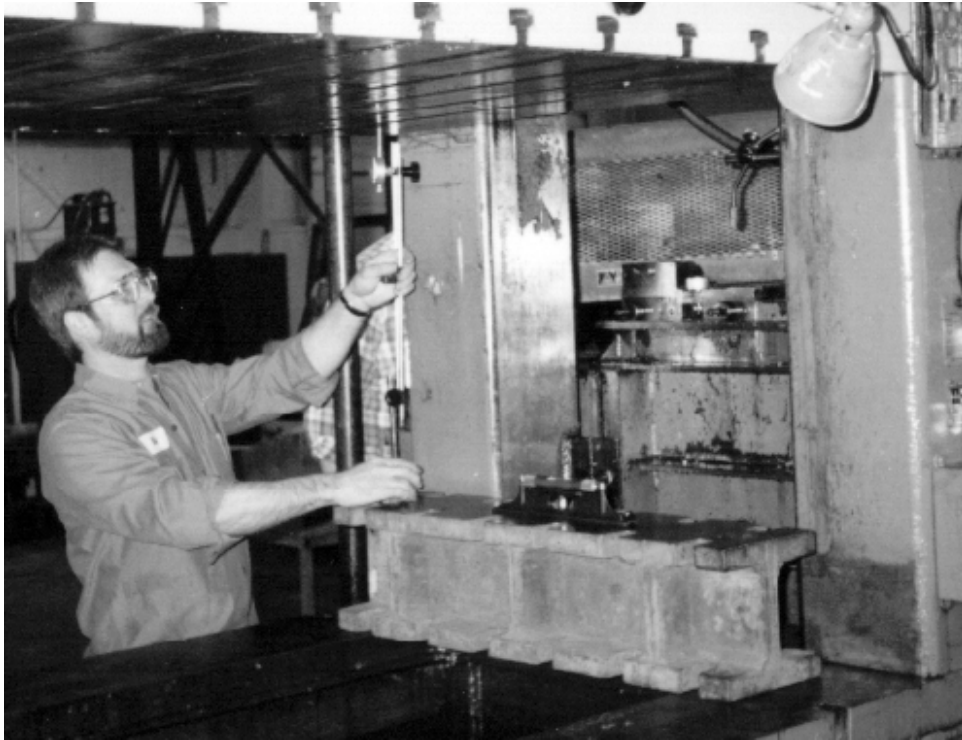
Figure 3. A maintenance technician checking a straightside presses for parallelism of the slide with the bed with a dial indicator. Note that the bolster is removed to eliminate a source of inaccuracy and a machinist's level is placed on the iron die parallel.
