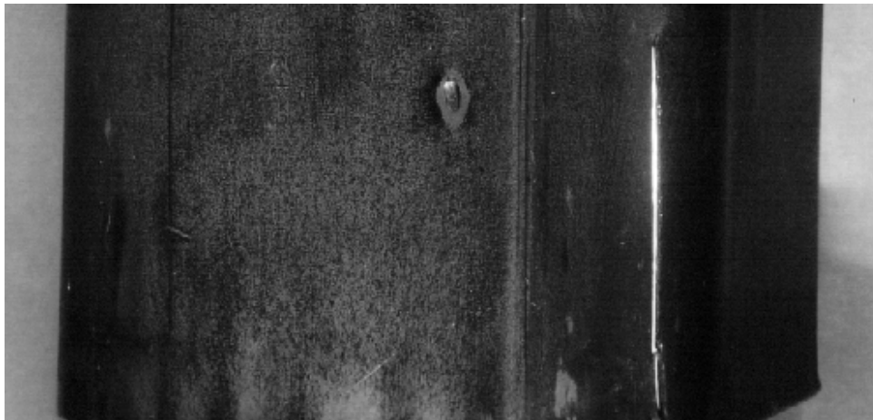
Figure 15. This photograph is taken with a powerful quartz halogen lamp inside a rectangular drawn shell. The intense light reveals a hairline crack—a serious defect. The crack occurs when a joggle to the left of the crack is formed. Smith & Associates
