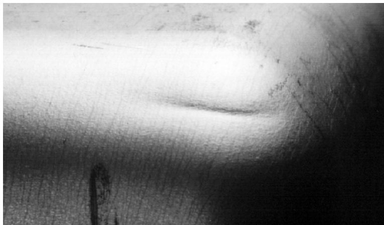
Figure 4. Photograph of a necking failure on the corner of a deep drawn box shaped stamping. Smith & Associates
